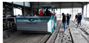
Freewalk barn with sand bedding (Free-Living Barn) and BeddingCleaner that picks up feces from sand bedding
